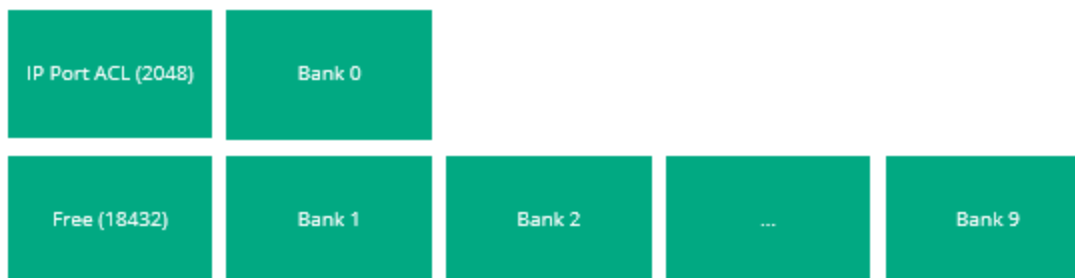
Figure 2 One bank reservation
